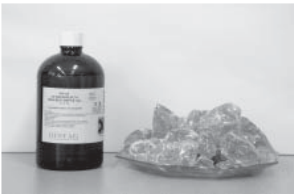
Fig. 7: Volatile and non-volatile pine gum fractions: turpentine oil and colophony
